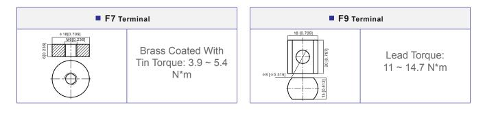
VALVE REGULATED LEAD-ACID BATTERY, RECHARGABLE
